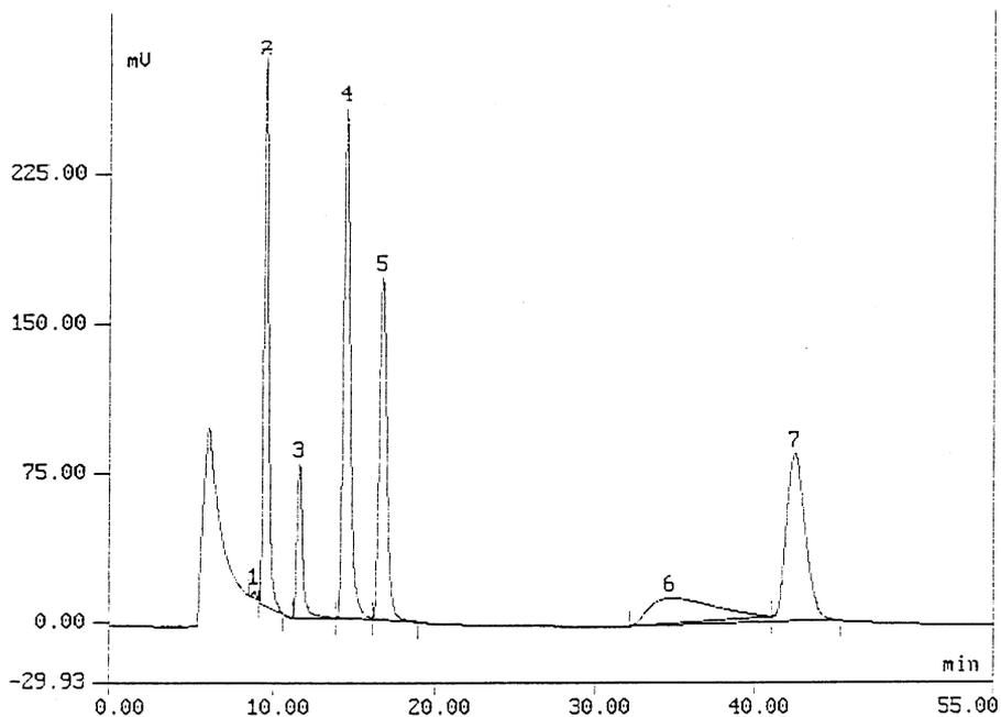
Fig. 2. Chromatogram of solution at 0.6 mM containing: GTP (1), IMP (2), uric acid (3), hypoxanthine (4), xanthine (5), adenine (6), and inosine (7). Mobile phase: 25 mM  $\text{NH}_4\text{H}_2\text{PO}_4$ , 1.5% methanol; pH 4.5; flow rate:  $0.5 \text{ ml h}^{-1}$ ; 1 mM corresponding at  $1 \times 10^{-3}$  absorbance; detection wavelength 254 nm.
